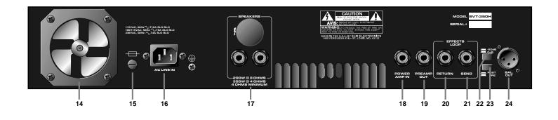
**14. FAN:** The temperature controlled, variable speed fan forces cool air into the amplifier, forcing heat out through the exhaust vents (also on the rear panel, between the speaker jacks and the power amp in jack). Never block the vent holes or the fan openings.
